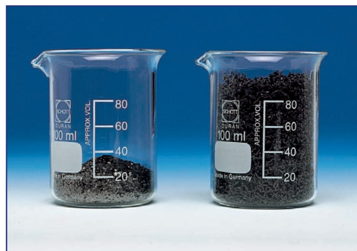
Graphite functions as a fire retardant due to its specific swelling effect.
