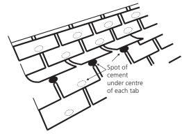
This procedure is especially recommended for all installations in high wind areas for the top five courses of shingles immediately below any roof ridge, which are usually most susceptible to wind uplift.
