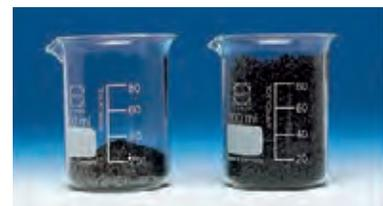
The swelling effect of graphite after exposure to fire can be seen in this comparison. Note the volume increase in the post-fired graphite in the beaker on the right.
