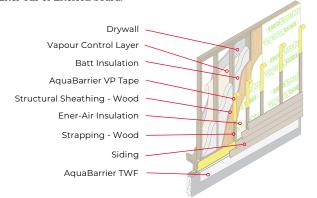
AcrylicStick SA Tapes and AquaBarrier VP Tapes are primerless and thus, require no adhesive. However, the AquaBarrier AVB Tapes must be adhered using IKO Adhesive primers³ (S.A.M. or S.A.M. LVC Adhesive). Any smaller penetration areas must be sealed using AquaBarrier Mastic.
