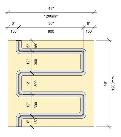
**INSULATION ADHESIVE BEAD PATTERN,** 4'X 4' BOARD, 12" ROWS
