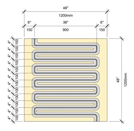
INSULATION ADHESIVE BEAD PATTERN, 4'X 4' BOARD, 4" ROWS
