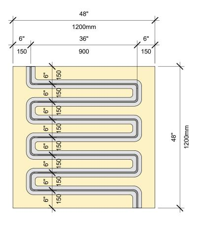
INSULATION ADHESIVE BEAD PATTERN, 4'X 4' BOARD, 6" ROWS
