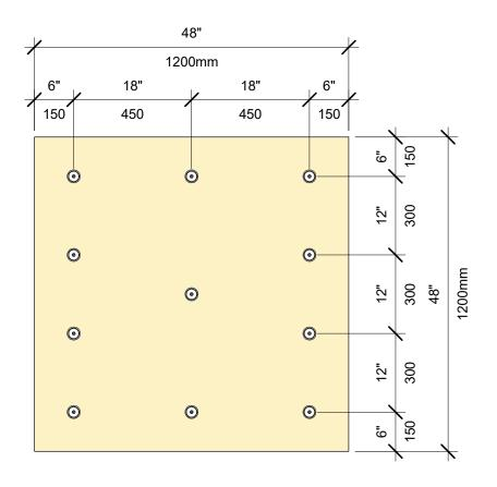
SCHÉMA DE FIXATION POUR ISOLATION: PANNEAU DE 4 PI SUR 4 PI, 11 FIXATIONS
