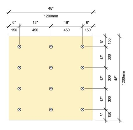
SCHÉMA DE FIXATION POUR ISOLATION: PANNEAU DE 4 PI SUR 4 PI, 12 FIXATIONS
