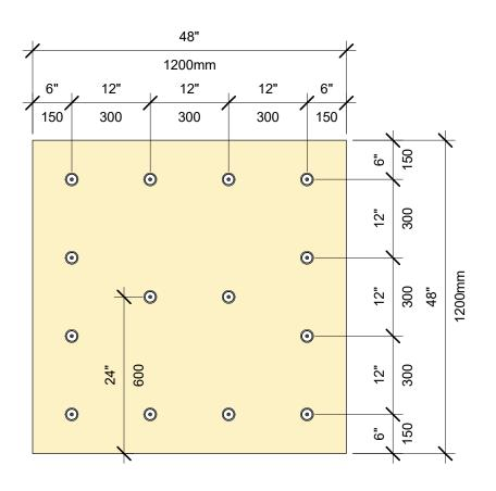
SCHÉMA DE FIXATION POUR ISOLATION: PANNEAU DE 4 PI SUR 4 PI, 14 FIXATIONS
