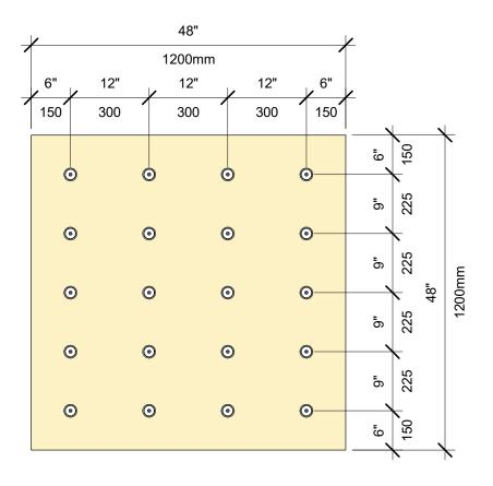
SCHÉMA DE FIXATION POUR ISOLATION: PANNEAU DE 4 PI SUR 4 PI, 20 FIXATIONS
