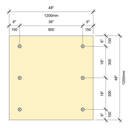
SCHÉMA DE FIXATION POUR ISOLATION: PANNEAU DE 4 PI SUR 4 PI, 6 FIXATIONS
