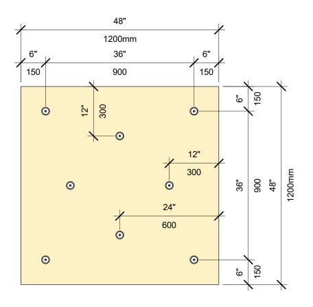
SCHÉMA DE FIXATION POUR ISOLATION: PANNEAU DE 4 PI SUR 4 PI, 8 FIXATIONS
