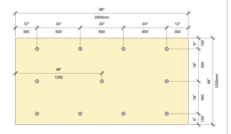
SCHÉMA DE FIXATION POUR ISOLATION: PANNEAU DE 4 PI SUR 8 PI, 11 FIXATIONS
