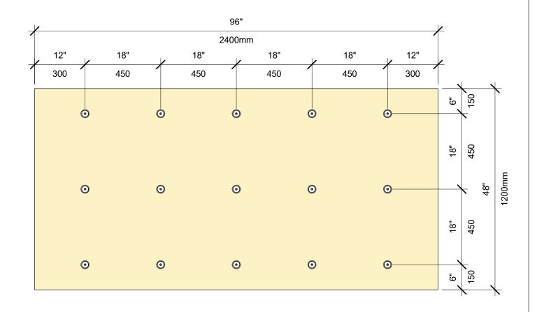
SCHÉMA DE FIXATION POUR ISOLATION: PANNEAU DE 4 PI SUR 8 PI, 15 FIXATIONS
