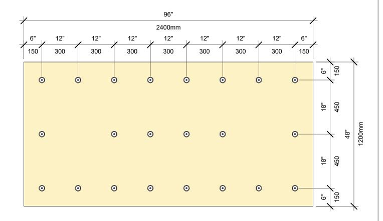
SCHÉMA DE FIXATION POUR ISOLATION: PANNEAU DE 4 PI SUR 8 PI, 22 FIXATIONS
