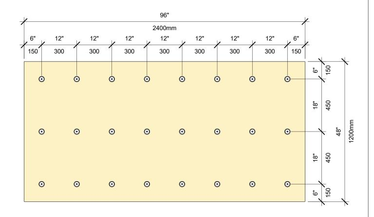
SCHÉMA DE FIXATION POUR ISOLATION: PANNEAU DE 4 PI SUR 8 PI, 24 FIXATIONS
