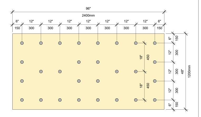
SCHÉMA DE FIXATION POUR ISOLATION: PANNEAU DE 4 PI SUR 8 PI, 28 FIXATIONS
