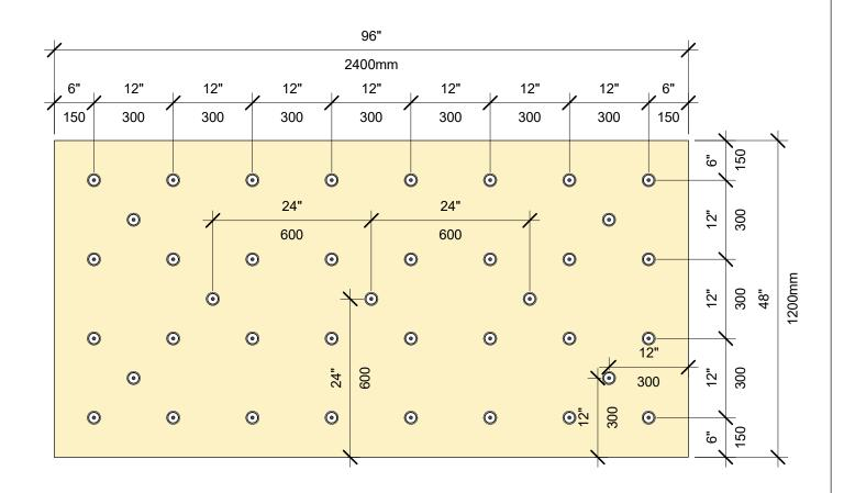
SCHÉMA DE FIXATION POUR ISOLATION: PANNEAU DE 4 PI SUR 8 PI, 39 FIXATIONS
