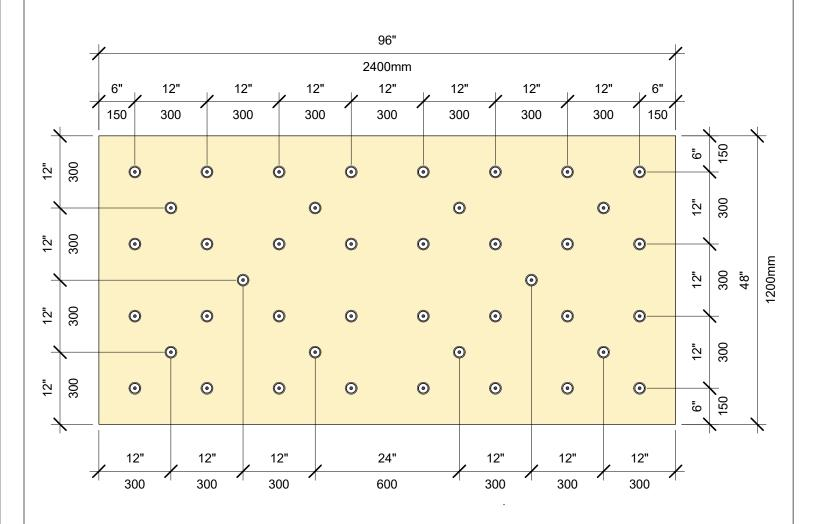
SCHÉMA DE FIXATION POUR ISOLATION: PANNEAU DE 4 PI SUR 8 PI, 42 FIXATIONS
