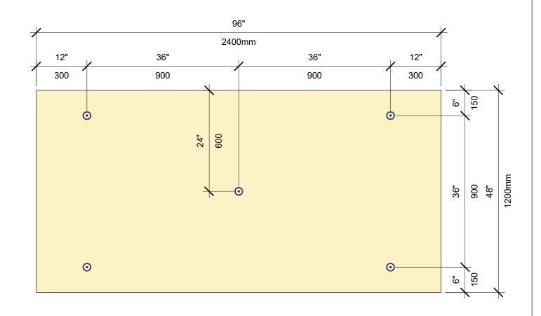
SCHÉMA DE FIXATION POUR ISOLATION: PANNEAU DE 4 PI SUR 8 PI, 5 FIXATIONS
