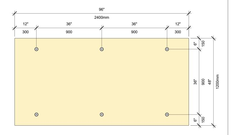
**SCHÉMA DE FIXATION POUR ISOLATION: PANNEAU DE 4 PI SUR 8 PI, 6 FIXATIONS**
