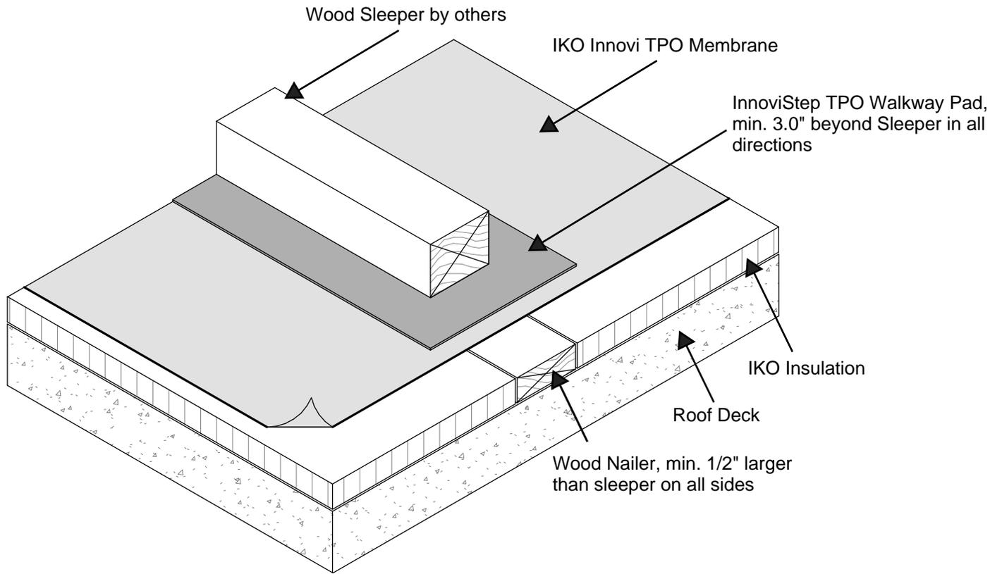
Sleepers bearing loads less than 5 lbs/in<sup>2</sup> (3.5 kg/mm<sup>2</sup>) do not require a wood nailer support.
