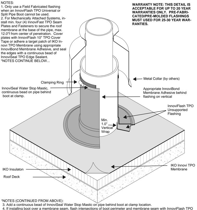
4. If installing boot over a membrane seam, flash intersections of boot perimeter and membrane seam with InnoviFlash TPO Joint Covers.
