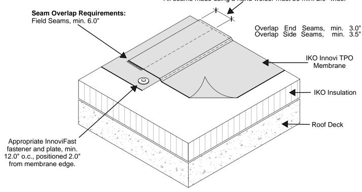
Apply InnoviSeal TPO Edge Sealant at all cut or exposed membrane edges
