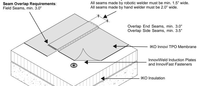
Apply InnoviSeal TPO Edge Sealant at all cut or exposed membrane edges
