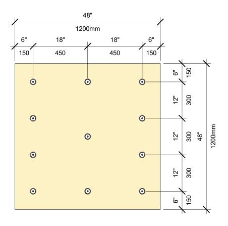
INSULATION FASTENING PATTERN: 4' X 4' BOARD, 11 FASTENERS
