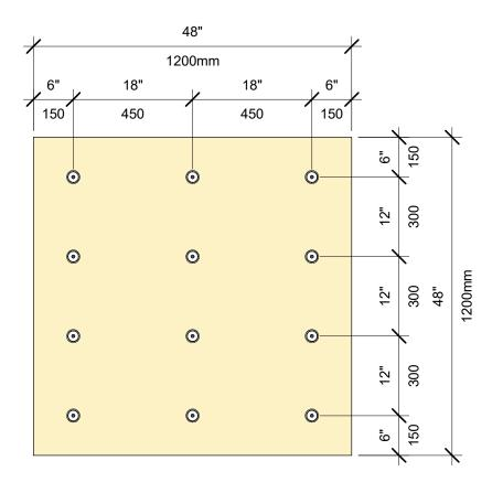
INSULATION FASTENING PATTERN: 4' X 4' BOARD, 12 FASTENERS
