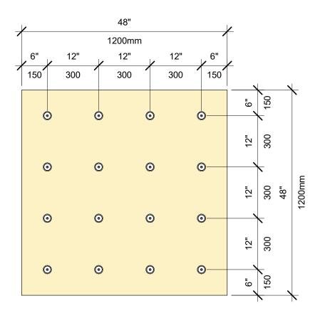
INSULATION FASTENING PATTERN: 4' X 4' BOARD, 16 FASTENERS
