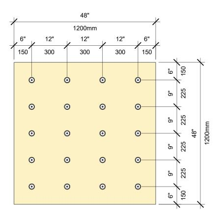
INSULATION FASTENING PATTERN: 4' X 4' BOARD, 20 FASTENERS
