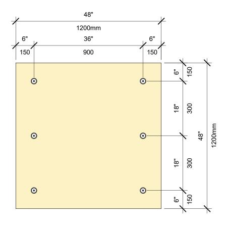
**INSULATION FASTENING PATTERNS:** 4' X 4' BOARD, 6 FASTENERS
