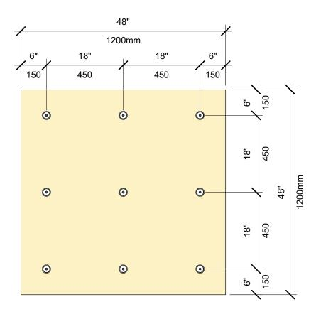
INSULATION FASTENING PATTERN: 4' X 4' BOARD, 9 FASTENERS
