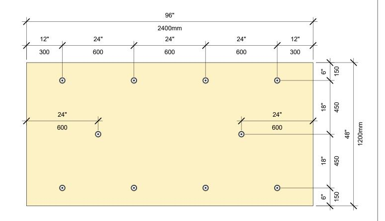
**INSULATION FASTENING PATTERN** 4' X 8' BOARD, 10 FASTENERS
