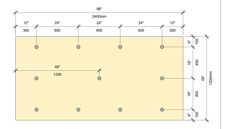
**INSULATION FASTENING PATTERN** 4' X 8' BOARD, 11 FASTENERS
