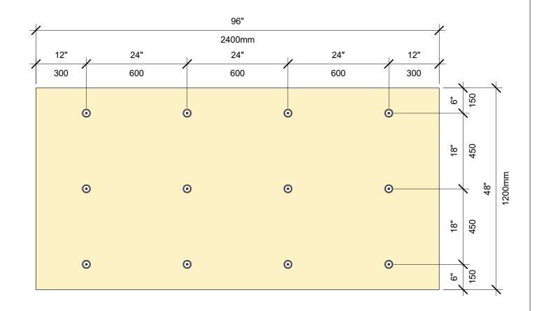
**INSULATION FASTENING PATTERN** 4' X 8' BOARD, 12 FASTENERS
