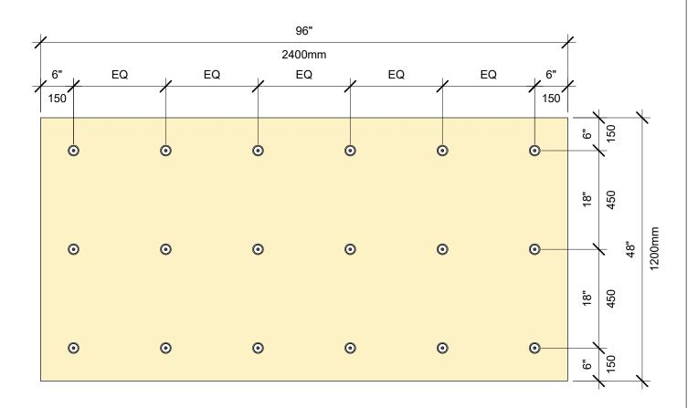
INSULATION FASTENING PATTERN 4' X 8' BOARD, 18 FASTENERS
