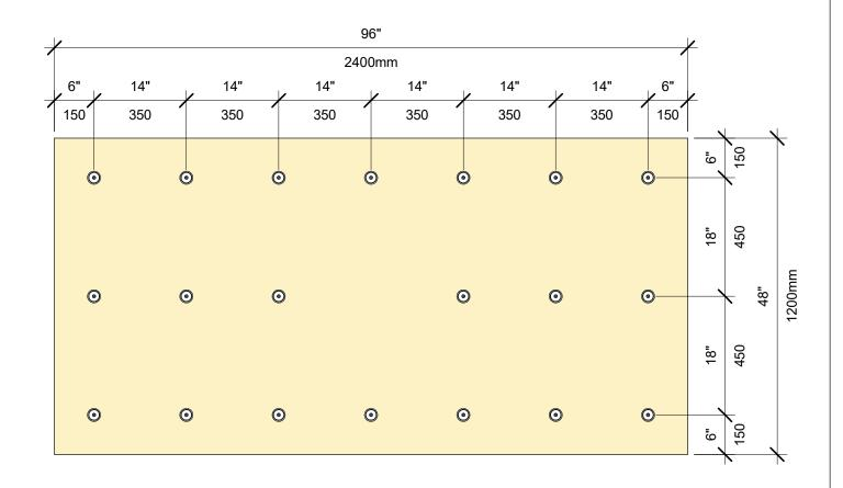
INSULATION FASTENING PATTERN 4' X 8' BOARD, 20 FASTENERS
