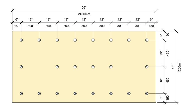
INSULATION FASTENING PATTERN 4' X 8' BOARD, 22 FASTENERS
