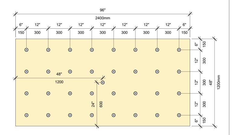
INSULATION FASTENING PATTERN 4' X 8' BOARD, 33 FASTENERS
