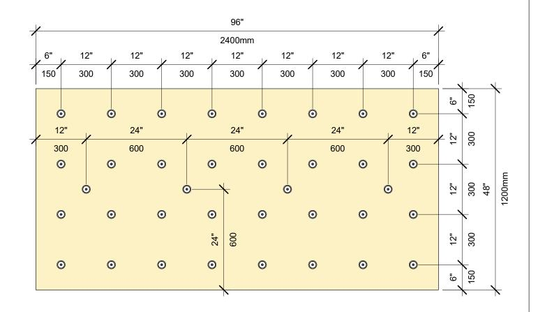
INSULATION FASTENING PATTERN 4' X 8' BOARD, 36 FASTENERS
