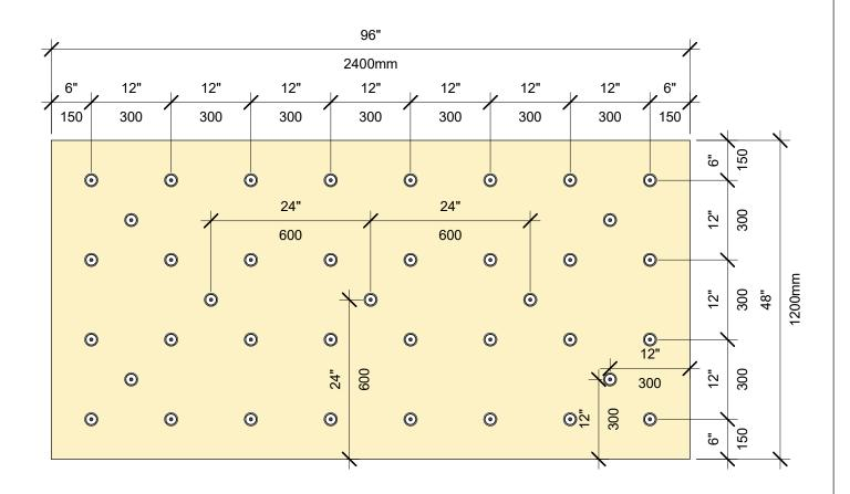
INSULATION FASTENING PATTERN 4' X 8' BOARD, 39 FASTENERS
