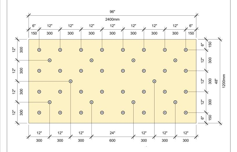
INSULATION FASTENING PATTERN 4' X 8' BOARD, 42 FASTENERS
