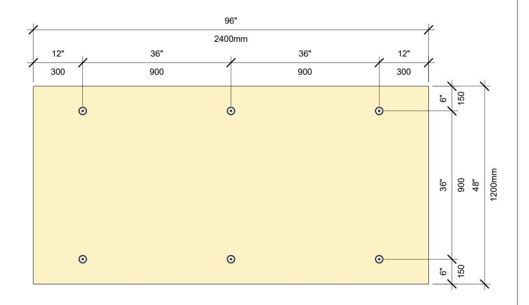
**INSULATION FASTENING PATTERN:** 4' X 8' BOARD, 6 FASTENERS
