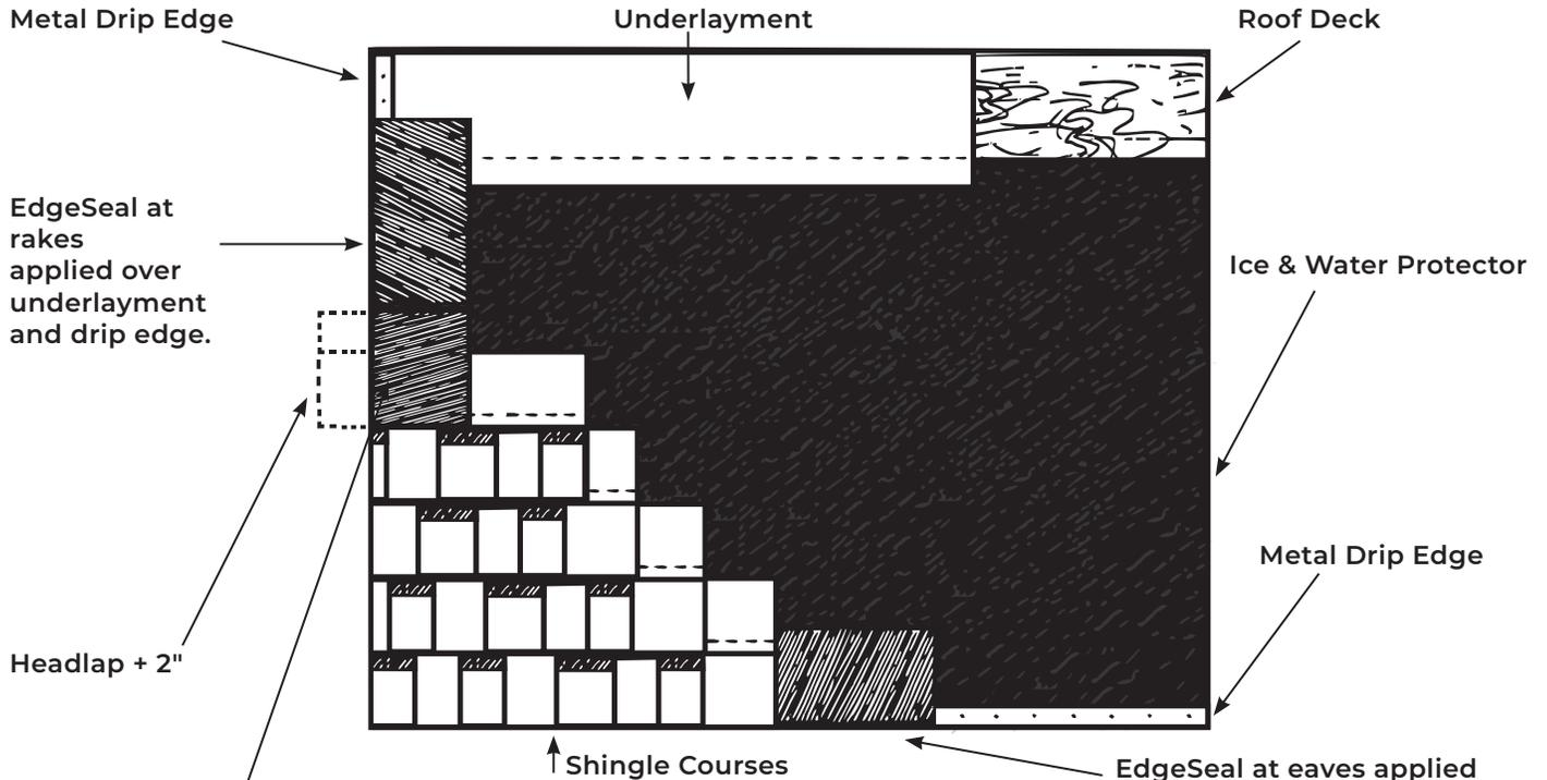
Apply EdgeSeal at headlap to seal rake edge exposure. Extend EdgeSeal at least 2" beyond the headlap going up the slope.
