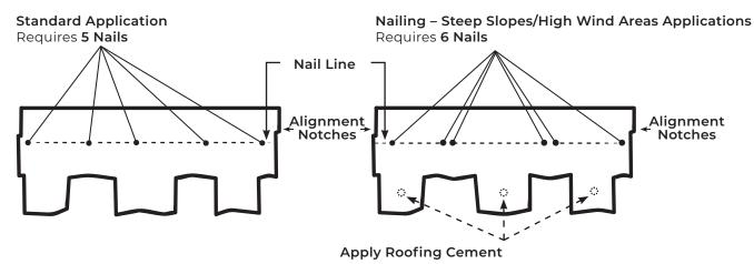
CAUTION: Excessive Use of Roofing Cement Can Cause Shingles to Blister.
