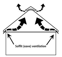
Ventilation should be balanced with 50% at the intake on the eaves or soffits and 50% on the ridge
