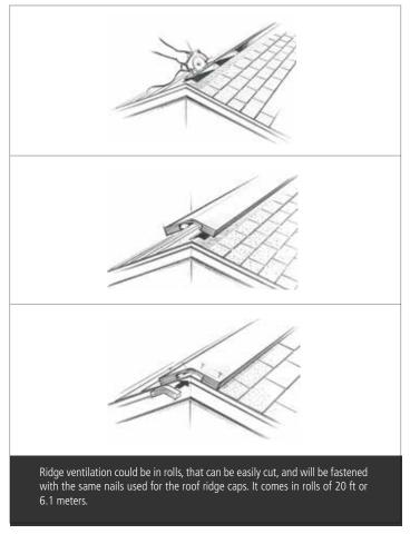
Reviewing this example, this roof of 60  $m^2$  of attic floor, will need 310 square inches of NFA of ventilation.
