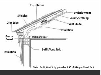
THERMALLY INSULATED ROOFS must have a ventilation channel at least 4 to 6 cm between deck and insulation.
