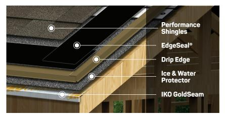
Detail A: Installation Diagram for Eaves and Rakes
