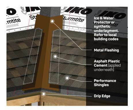
Detail D: EdgeSeal Installation Diagram for Valley
