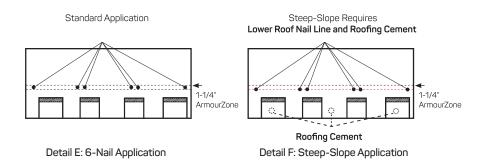
After installing the first shingle in the course, continue with full-length shingles to complete the first course and trim the last shingle so that it matches the overhang of the EdgeSeal, of 1/4 inch to 3/4 inch.
