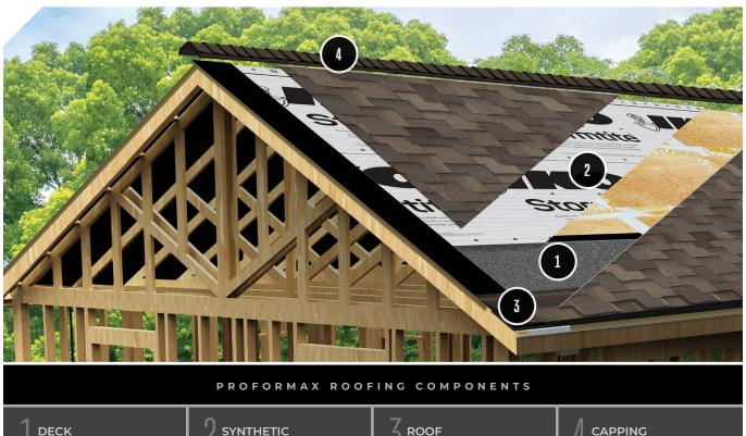
1 DECK PROTECTION 2 SYNTHETIC UNDERLAYMENT 3 ROOF STARTERS 4 CAPPING SHINGLES
