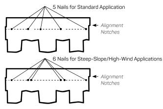
Shingles must be installed according to all of IKO's application instructions. Some select installation requirements are highlighted here.
