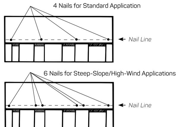
Shingles must be installed according to all of IKO's application instructions. Some select installation requirements are highlighted here.
